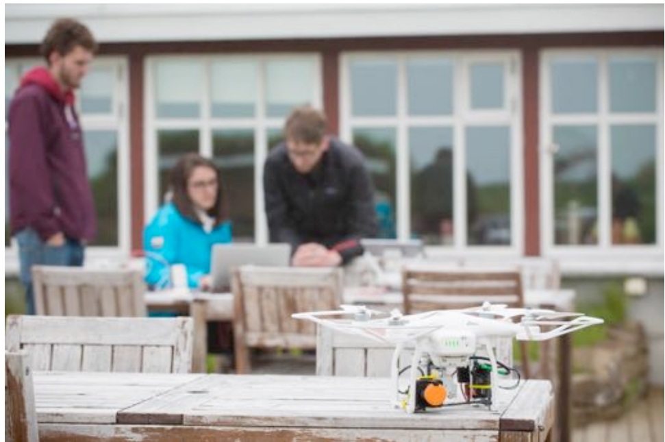
Figure 15. The orange and black unit is the LiDAR platform, the compute board is to the right of it.
