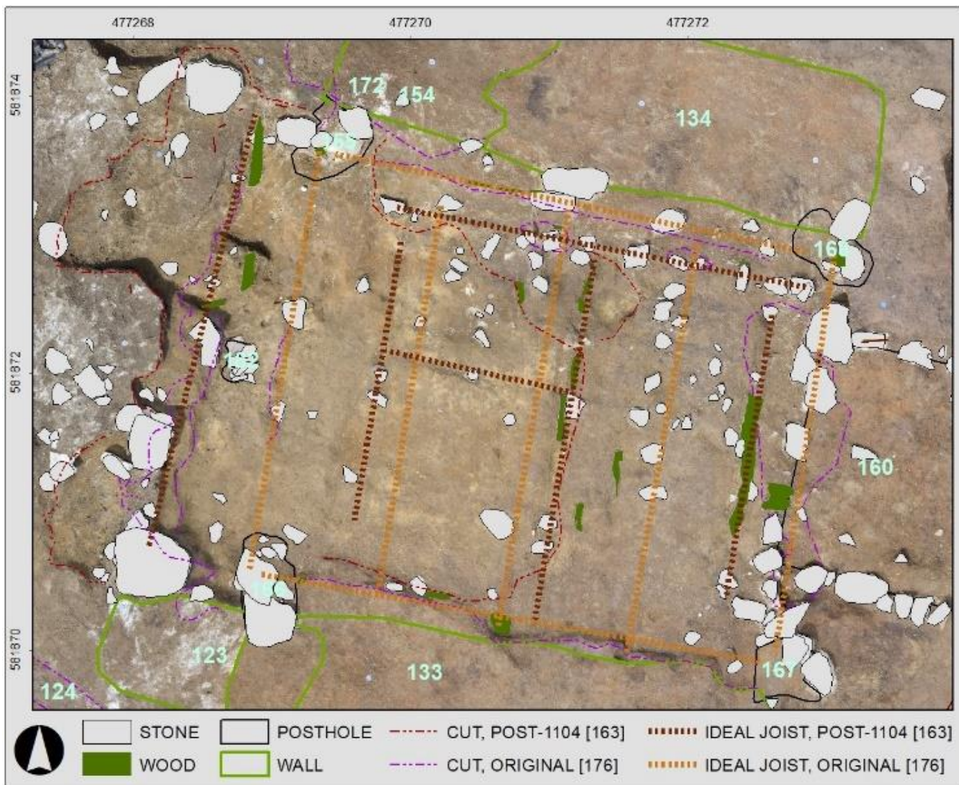
Figure 23. Foundations cuts in the church and hypothesized location of original floor joists for the original church and post-1104 reconstruction.
